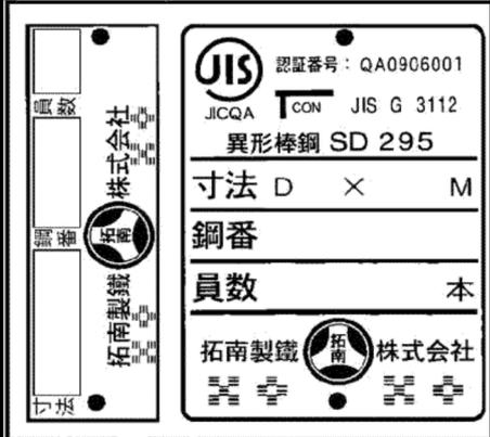
A white rectangular label with a black border. It contains the following text: JIS logo with certification number QA0906001, JICQA T CON JIS G 3112, 異形棒鋼 SD 295, 寸法 D × M, 鋼番, 員数 本, and 拓南製鐵 株式会社 logo at the bottom. On the left side, there is a vertical stamp area with the text 拓南製鐵 株式会社 and a circular logo. |
